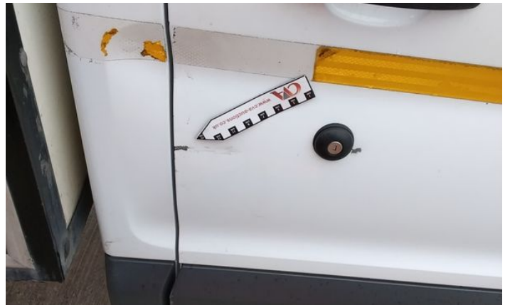
4: Door nsf Rusted Over 5mm
